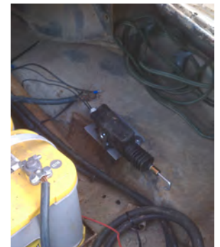
The door lock actuator Steve utilized to pull the parachute release cable.
