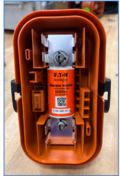
Figure 3: High-voltage battery disconnect from a Chevrolet Bolt
